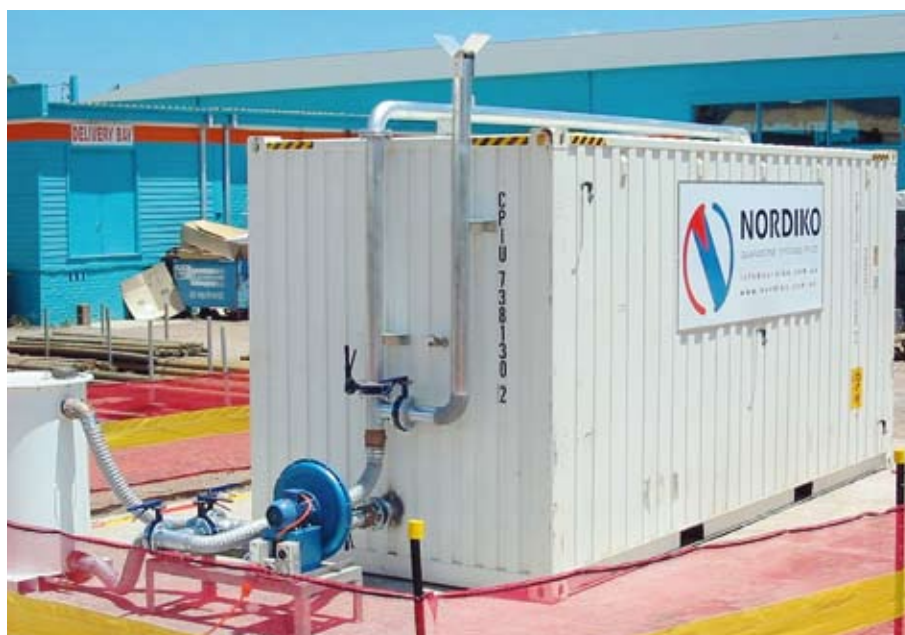
Recapture of methyl bromide on a freight container (Nordiko)
